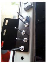
Next put the template on the plastic A pillar trip, drill two 6mm holes and cut between them with the dremel. give it a file and put it back on the A pillar over the mounting bracket.
