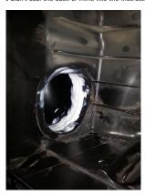
This hole i sealed from the bottom. possibly didnt need it, when the engine is running the sucking air should close it and seal it, but i wasn't taking any chances.
