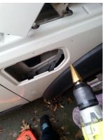
Now remove the plastic cover panel on the front A pillar. install the template, mark and punch the holes. This is a pain in the ass. The first skin is easy to drill through. the second skin takes ages. Use the 5mm cobalt drill bits and the side handle on the drill, and just keep going. don't go too fast as you don't want to heat up and harden the steel, but don't go to slow cuz it takes ages. I changed drill bits every 2 holes. don't know if it helped or not.
